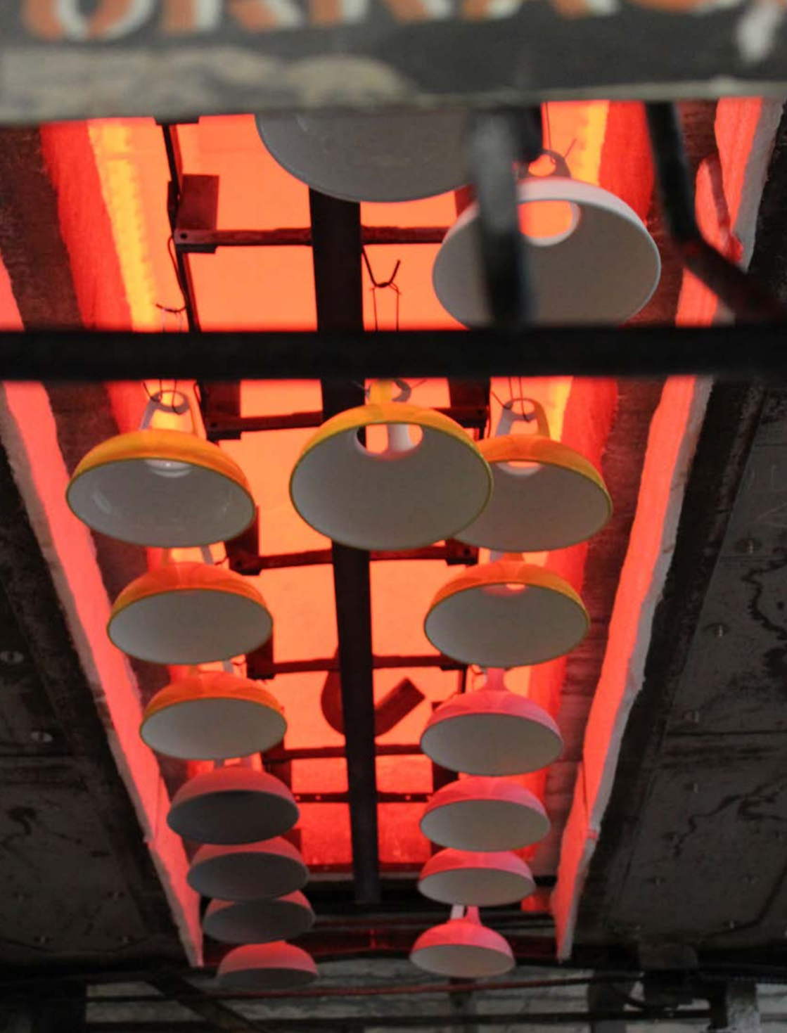
Firing of the white inside, the final one after building up the outside coat
